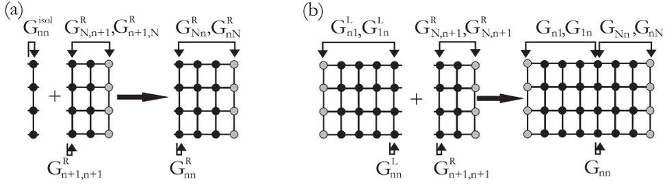
**Figure 4.5:** Extension of the standard recursive technique. The isolated columns are glued together, but now starting from the righthand side (a). The final step consists of adding these strips of columns to the ones calculated in Fig. 4.4 (b).
